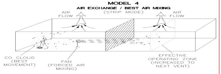
Notice the CO concentration and the Effective Operating Zone (Expanded through the Dividing zone to the second vent) with air exchange and forced air mixing through the dividing Zone. The CO cloud is diluted with the available air in the building. Note the "Dividing Zone" shown above, this is the line where airflow changes direction. In Model 4, air changes are full as forced air mixing has moved and mixed the CO between all air zones.
