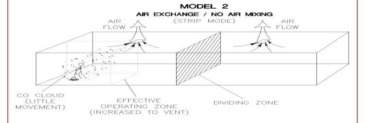
• Notice the CO concentration and the Effective Operating Zone with air exchange. The CO cloud is still concentrated in a small area. Note the "Dividing Zone" shown above, this is the line where airflow changes direction. In Model 2, air changes are cut in ½ as little or no CO crosses the Dividing Zone to be exhausted.
