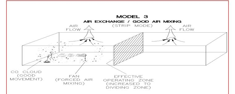
• Notice the CO concentration and the Effective Operating Zone (Expanded to the Dividing zone) with air exchange and forced air mixing with use of a fan. Placing of 4 large CFM fans in each corner of the work zone is most effective. The CO cloud is still concentrated on one side of the Dividing zone. Note the "Dividing Zone" shown above, this is the line where airflow changes direction. In Model 3, air changes are cut in ½ as little or no CO crosses the Dividing Zone to be exhausted.
